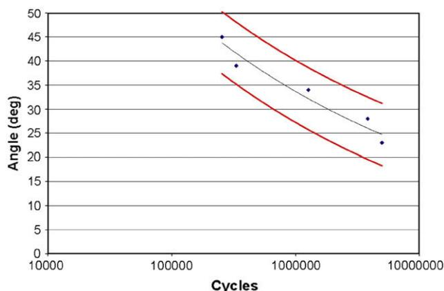
Fig. 3. Fatigue curve for dynamic compression bending results.
